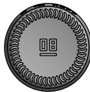
VIEW ON BASE SHOWING EMBOSSED MARKINGS & STANDING AREA EMBOSSED WITH STIPPLES.
